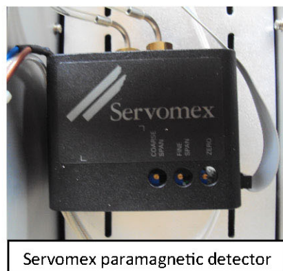
Internal view of GAS 3070 R PMGO 2 with SERVOMEX detector integrated in a temperature controlled enclosure
